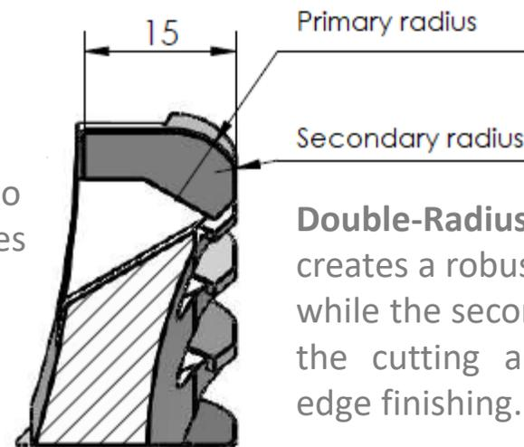
**Double-Radius.** The primary radius creates a robust profile for hogging, while the secondary radius protects the cutting area responsible for edge finishing.
